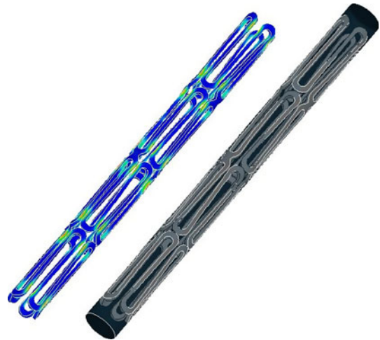
Fig. 2 The compression response of the parent device; fringe plot showing maximum principal strains on the left
